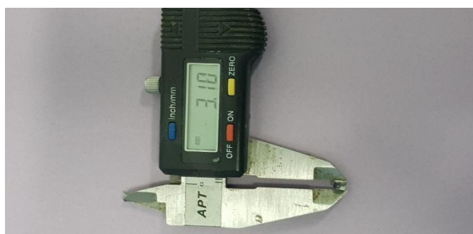
Figure 22. Using digital calibration tool to calibrate the thickness of each root section.
